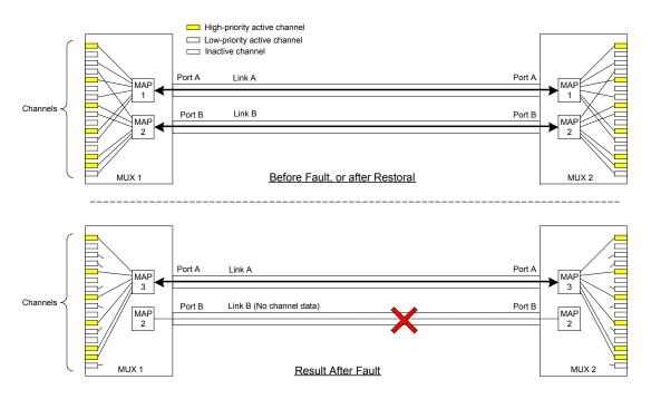
When both links are operational, channels may be assigned individually to either link, even up to the full composite bandwidth of that link. In this case, the resulting timeslot maps are constructed independently and contain no common channels.
