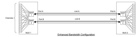
Two links are used for enhanced bandwidth, but it is not required that they be of equal rates. Channels are assigned individually to either of the two links. Should a link fault occur, the system will take no automatic action to recover or restore operation to the affected channels as long as the fault persists, other than to declare the appropriate fault alarm.
