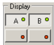
Fig. 5.4.1. – Channel visibility controls
